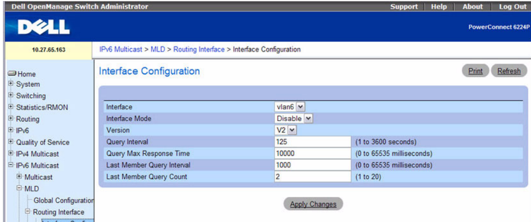
Figure 12-24. MLD Routing Interface Configuration
