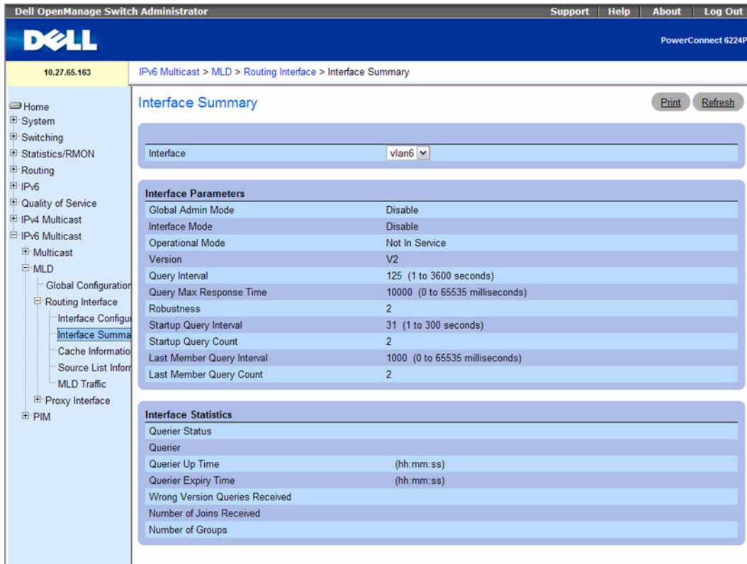
Figure 12-25. MLD Routing Interface Summary
